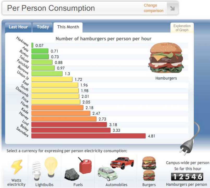
Figure 2: Online Comparison Tools for Evaluating Dormitory Energy Consumption. Oberlin's CRMS puts resource consumption in terms everyone can understand – whether that means Watts or Gallons, Dollars or Euros, Hamburgers or Veggie Burgers, lbs CO 2 or SUV miles driven.
