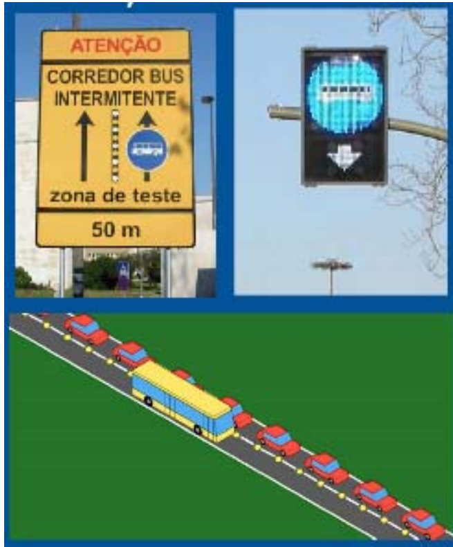
Figure 1: Signs Used in the Lisbon IBL. An explanatory sign (top right) tells drivers to look for signs indicating a change from a “regular lane” to a “bus lane.” When a bus is approaching in an IBL, the vertical traffic sign (top left) indicates that the lane has changed to a bus lane, while lights between the IBL and other traffic lanes (bottom) turn on to signal to cars that entering the IBL is not permitted.
