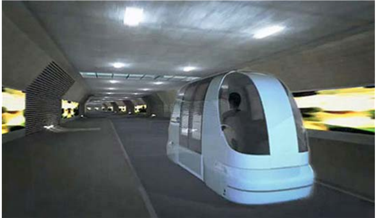
Figure 2: Masdar PRT System. An underground modular public transportation system with a central control system will give Masdar residents the convenience of a personal vehicle as well as the health and community benefits of car-free streets. The battery-powered PRT pods, shown above, hold up to six passengers. (Photo from http://www.inhabitat.com )
