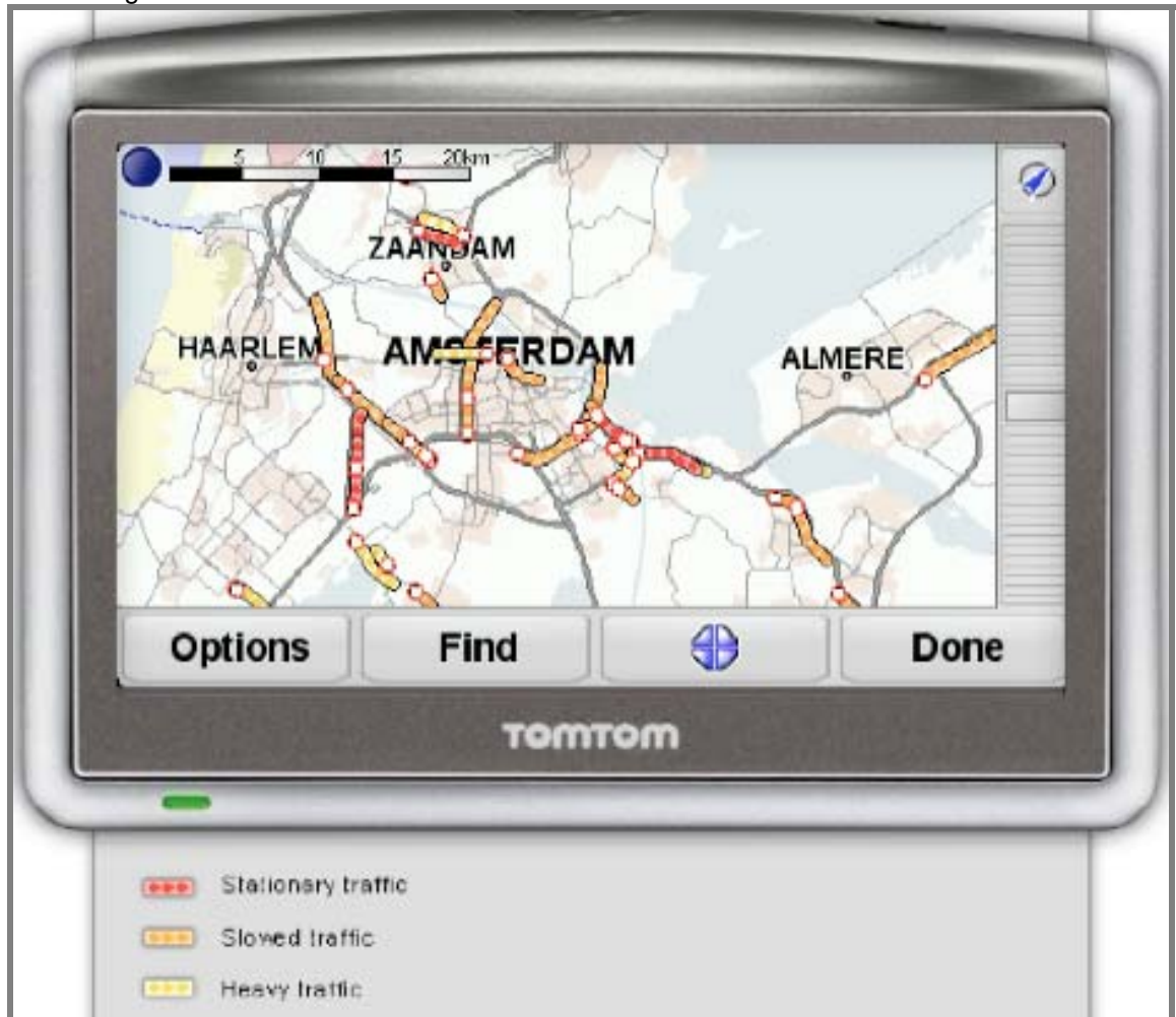
Figure 2: TomTom navigation system with Vodafone traffic information. While the TomTom-Vodafone partnership encounters fewer privacy concerns than the Mobile Century project, aggregate data collected from phone towers is less comprehensive and less precise than data collected directly from the phones themselves.
